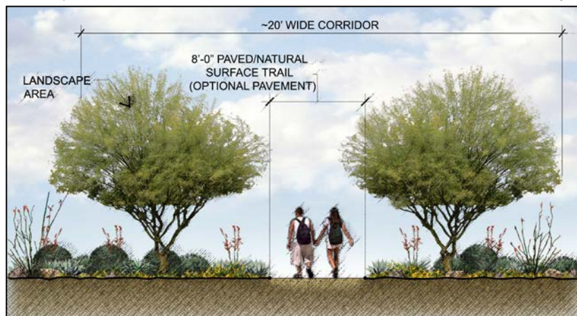
Figure 32: Local Area Trail Typical Cross-Section Detail
